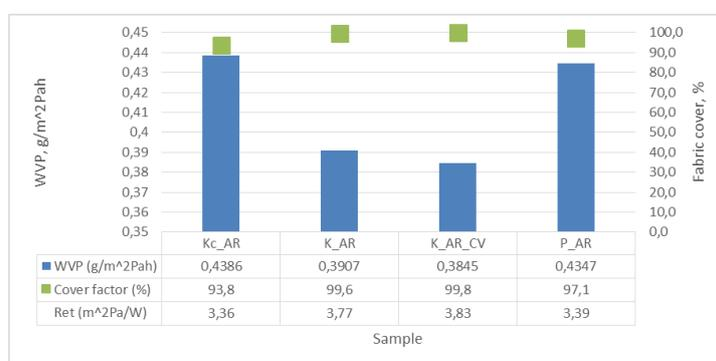
Figure 1. Water vapor permeability
