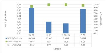
Figure 1. Water vapor permeability
