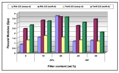
Figure 3. Influence of filler type and content on the flexural modulus of P/F hybrid biocomposites.
