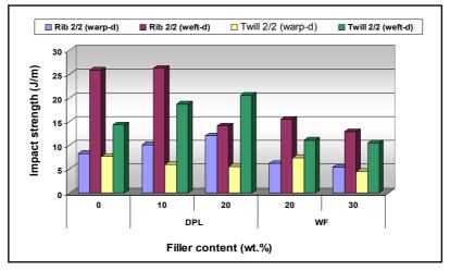
Figure 1. Influence of filler type and content on the impact strength of P/F hybrid biocomposites.
