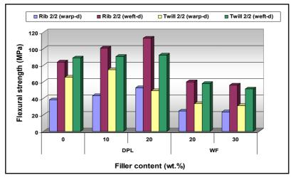
Figure 2. Influence of filler type and content on the flexural strength of P/F hybrid biocomposites.
