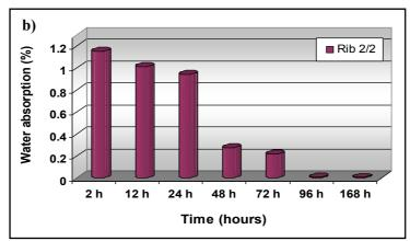
**Figure 5.** a) Influence of filler type and content on water absorption of P/F hybrid biocomposites after 168h, and b) water absorption rate of warp rib 2/2 biocomposites with adding 30% WF.
