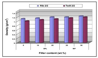
Figure 4. Influence of filler type and content on the density of P/F hybrid biocomposites.
