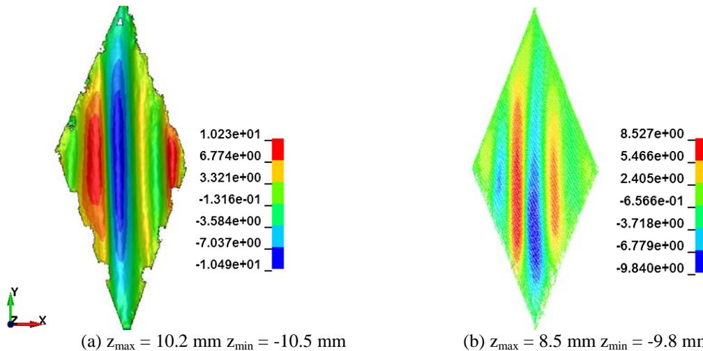
**Figure 8.** Optical comparison of the wrinkle size of fabrics variant 2 (a) Experiment (b) Simulation
