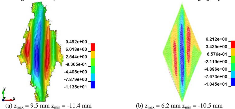
Figure 7. Optical comparison of the wrinkle size of fabrics variant 1 (a) Experiment (b) Simulation
