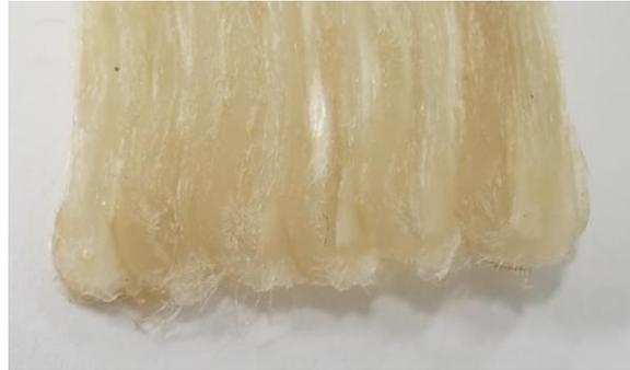
**Figure 3.** Tow pullup in regions of high path curvature.
