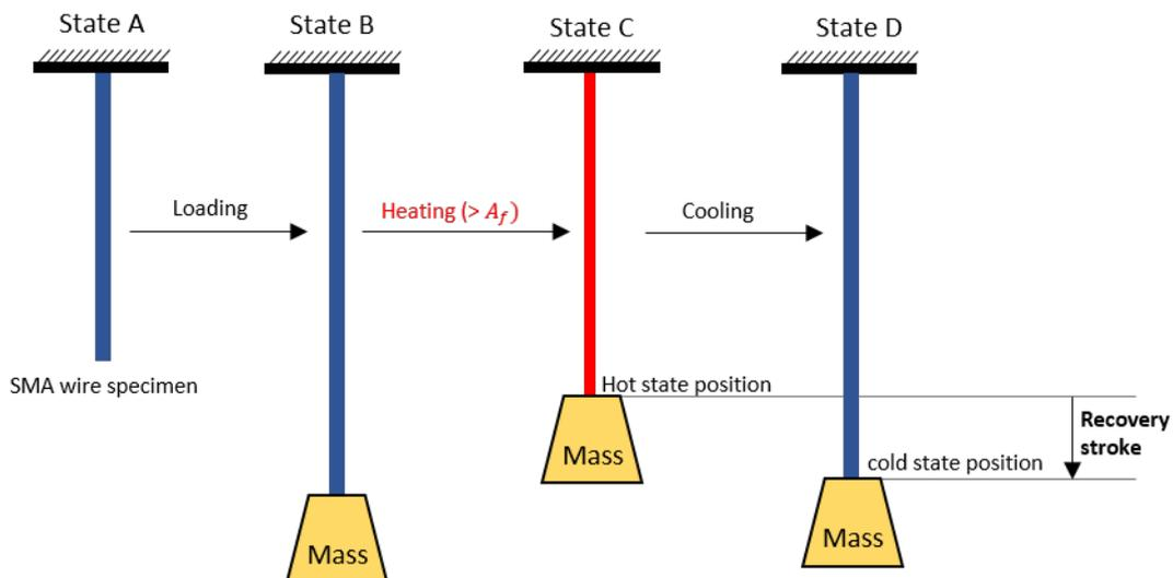
**Figure 1:** Concept of the Shape Memory Effect, based on [3]
