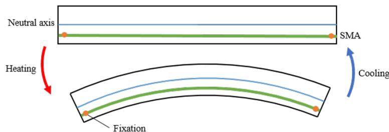
Figure 2. Bending beam principle [7]
