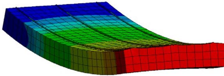
**Figure 4:** Model of elastomer bending beam with embedded SMA wires during thermal activation
