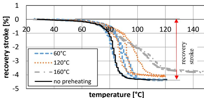
Figure 3: Reduction of SMA wire stroke after preheating with fixation
