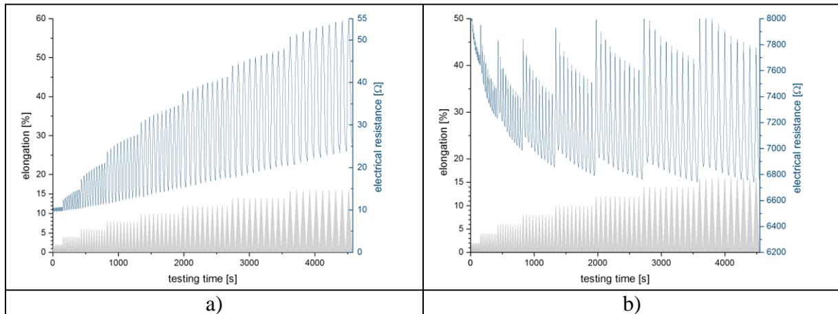
**Figure 3.** Results of electromechanical yarn characterization a) yarn T1 and b) yarn T2 (0 - 16 % elongation)
