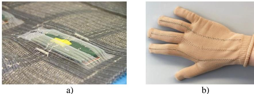
**Figure 2.** samples of textiles with integrated sensor yarn a) into a flat structure b) into a 3D-structure
