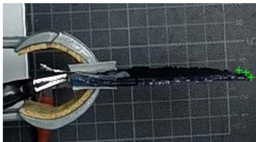
**Figure 3.** Tracking the displacements during actuation
