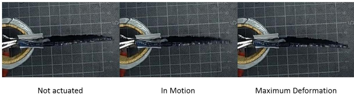
**Figure 4.** Fiber reinforced actuator when activated with 3kV
