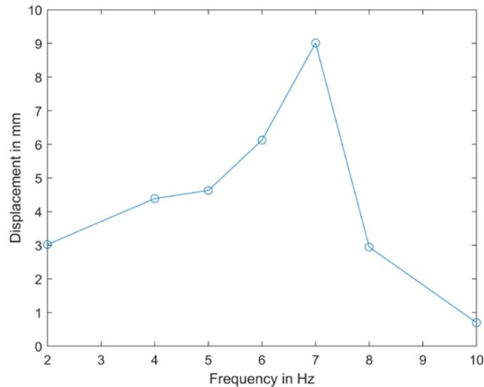
**Figure 6.** Displacement of the actuated bending beam for frequencies between 2 and 10 Hz
