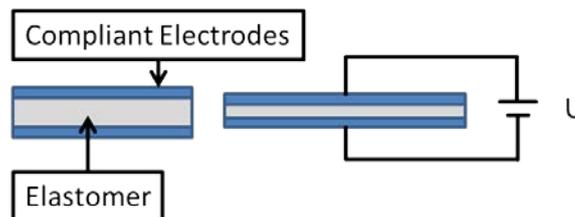
**Figure 1.** Mechanism of a dielectric elastomer actuator
