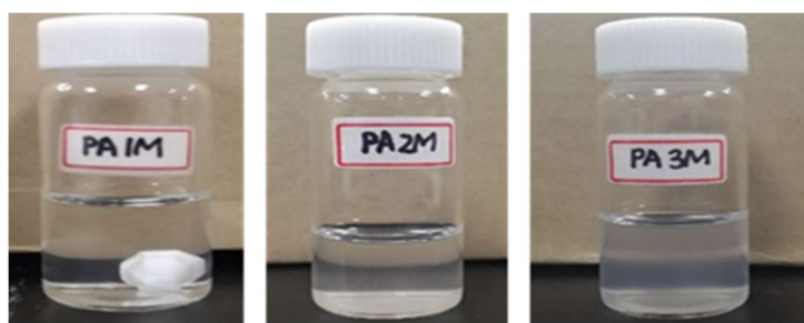
Figure 3. Aqueous ENC solutions prepared at different concentrations of PA at 80^{\circ}\text{C}
