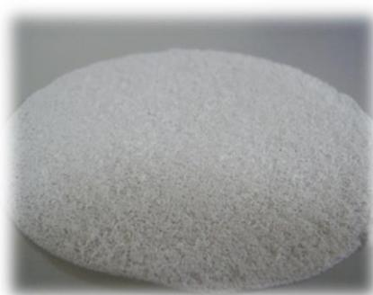
Figure 1. Manufactured porous material from acetyl-butyril chitin co-polyester (90/10) BAC and NaCl as the porophor agent in the membrane form [15]
