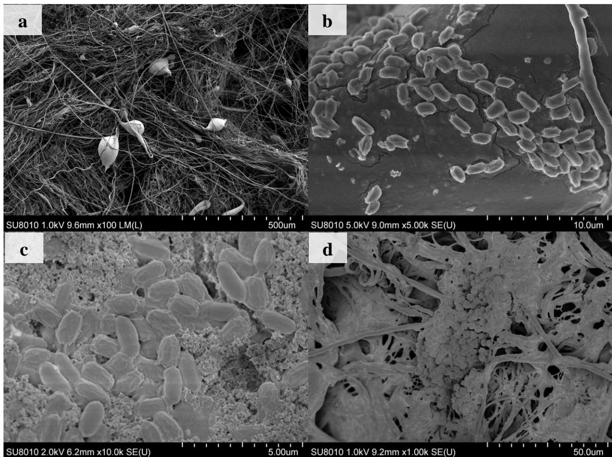
**Figure 2.** SEM images of (a) pristine melt-blown nonwoven (control sample) and (b-d) biofilms formed on dust-loaded nonwovens
