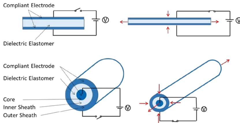
**Figure 1.** Working principle of a planar DEA and a DEA in filament form
