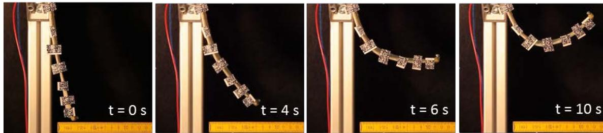
Figure 2. Movement of a SMA at different time intervals [3]
