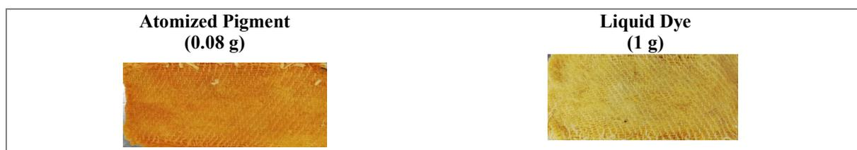
**Figure 2.** 100% Wool dyeing test Results with Bixin and Norbixina
