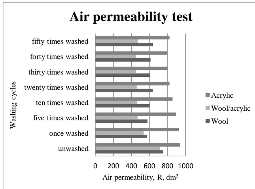
**Figure 1.** Air permeability of tested knitted fabrics
