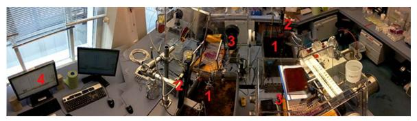
**Figure 1.** 180° bird eye view on the recent messy setup with: 1. Two incubated sediments (one aerated, one not), 2. profiling motors (Unisense, Denmark), 3. a glove box each with the pump and the fraction collector and 4. the evaluation units.
