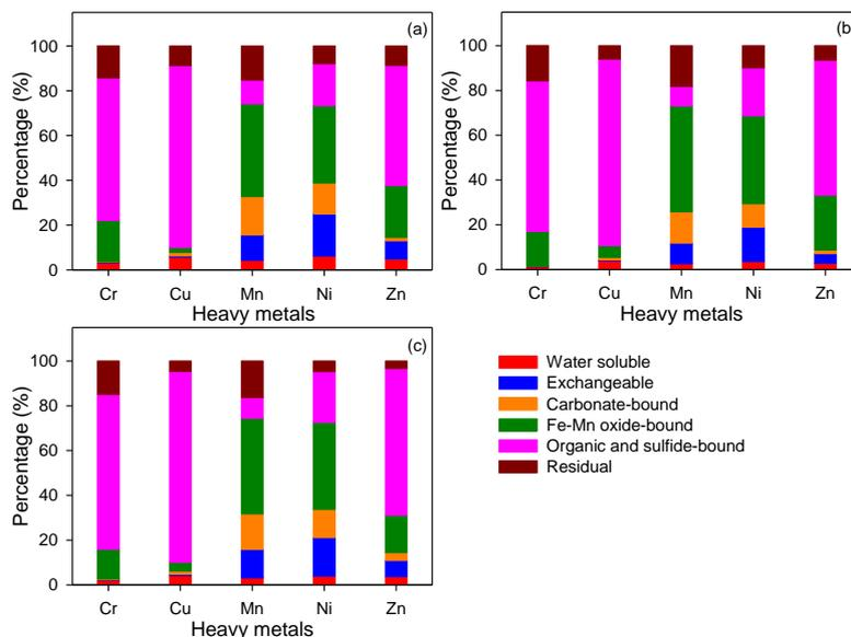
**Fig.1 Metals speciation in the solid phase of sludge after digestion R1 (a), R2 (b) and R3 (c)**
