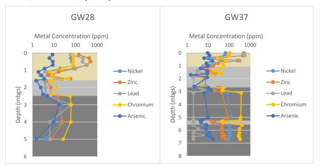
Figure 1. Plots of lithology and heavy metal distribution (Ni, Zn, Pb, Cr, As) against depth for GW28 and GW37.
