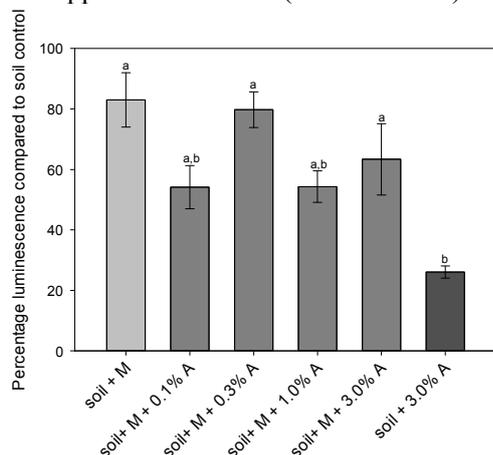
**Figure 1.** Bacterial biosensor toxicity tests of pore water for the different treatments (+M = with manure; + A = with ash). Bar represent the average of the replicates and the bar is the s.e.m (n=5). Means that share the same letter are not significantly different.
