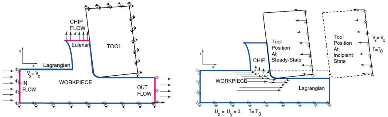
Figure 1. Finite element model for ALE formulation with: a) Eulerian and Lagrangian boundary conditions (with predefined chip) [11, 14], and b) pure Lagrangian boundary conditions [14].
