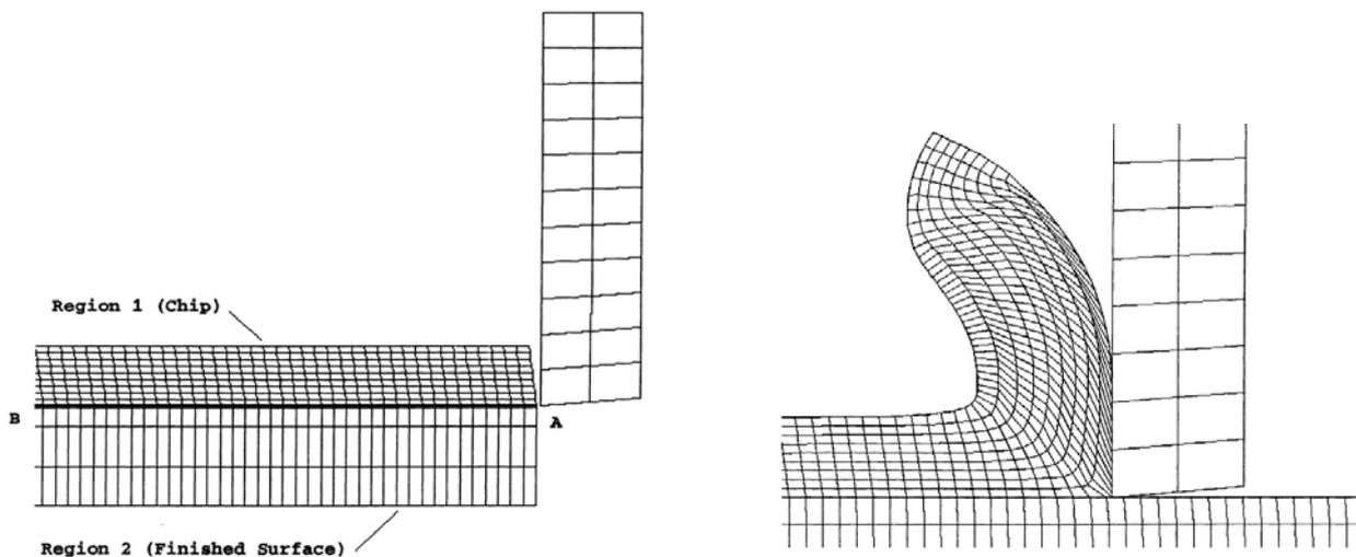
Figure 4. Left: Undeformed mesh with indication of node separation line (AB). Right: deformed mesh at steady-state cutting [7]
