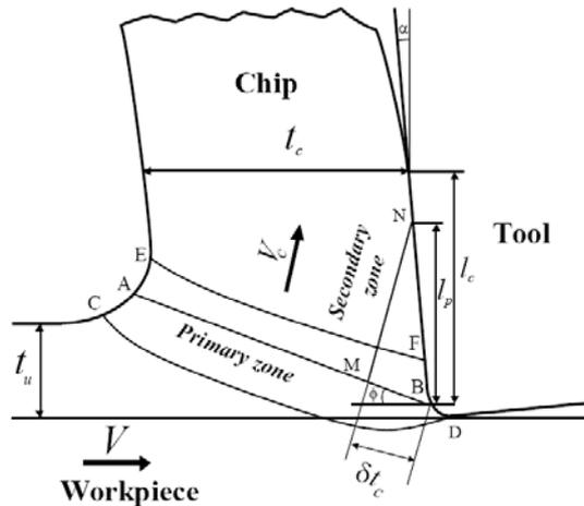
Figure 3. Parallel-sided shear zone model of Oxley [13].
