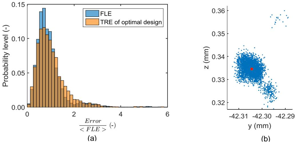
Figure 12: Error on one specific fiducial (Number 4). (a) TRE distribution of the target compared to the FLE distribution of one fiducial. This FLE has two maxima because of the non-normally distributed coordinates. (b) Y-z projected view of the measured points for fiducial 4.
