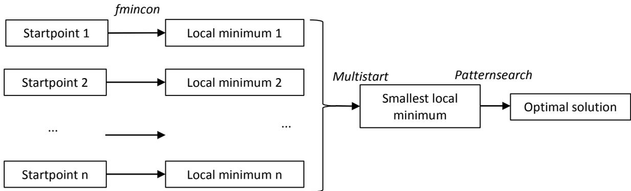
Figure 7: Flowchart of the optimisation function in Matlab
