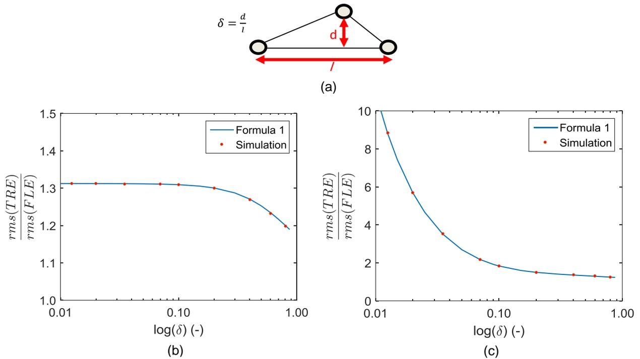
Figure 4: Influence of triangularity on TRE. (a) Definition of triangularity. (b) Starting from collinear fiducials and target point. (c) Starting from collinear fiducials and target point at 30 mm distance.
