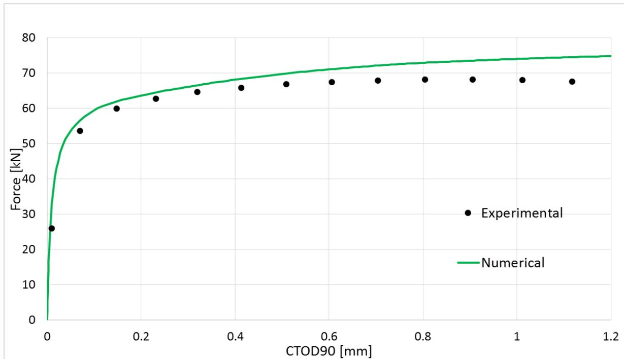
Figure 5: Experimental and numerical force versus CTOD<sub>90</sub> curve for the base material specimen
