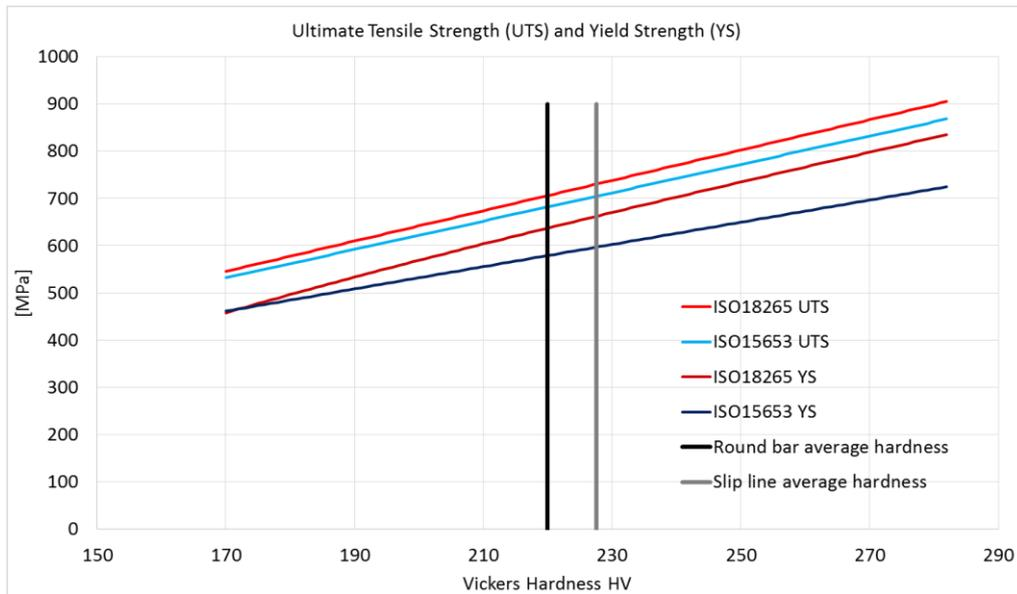
Figure 8: Ultimate tensile strength (UTS) and yield strength (YS) calculated from the ISO18265 (and FITNET-0.05) and ISO15653 standards based on the hardness range that occurs in the weld metal specimen.
