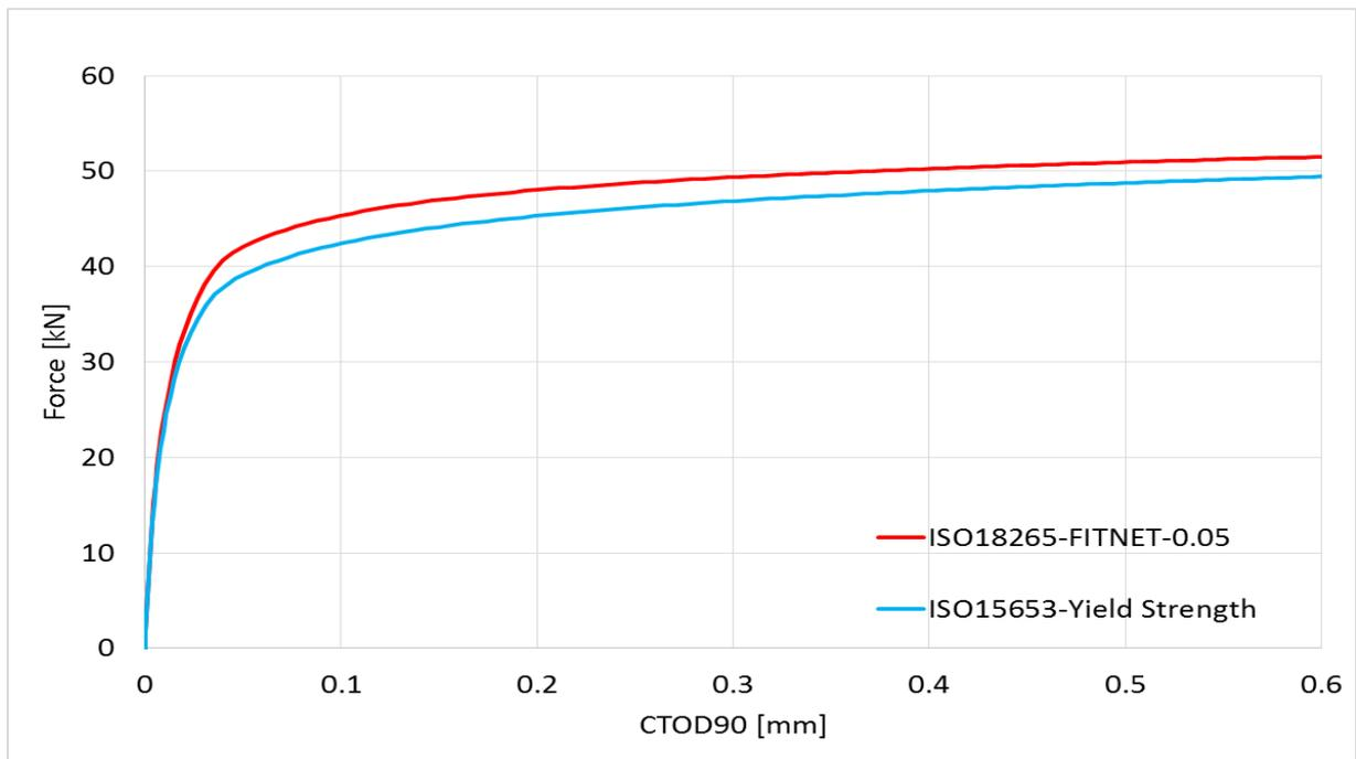
Figure 6: Force versus CTOD<sub>90</sub> simulation with two different transfer functions
