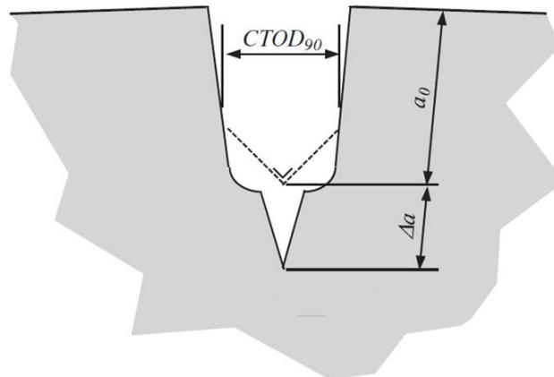
Figure 3: Schematic representation of  $CTOD_{90}$  for growing crack. [10]
