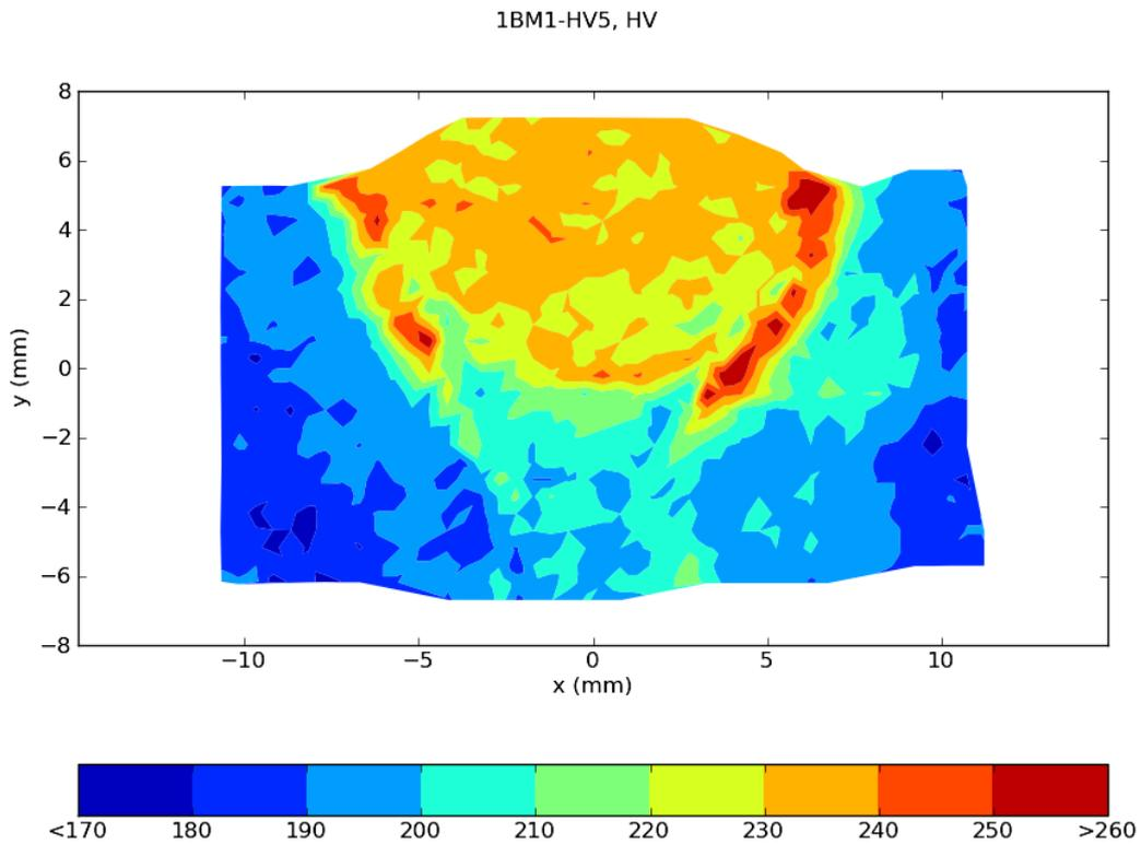
Figure 7: Hardness map of the weld from which the SENT specimen was extracted [9]
