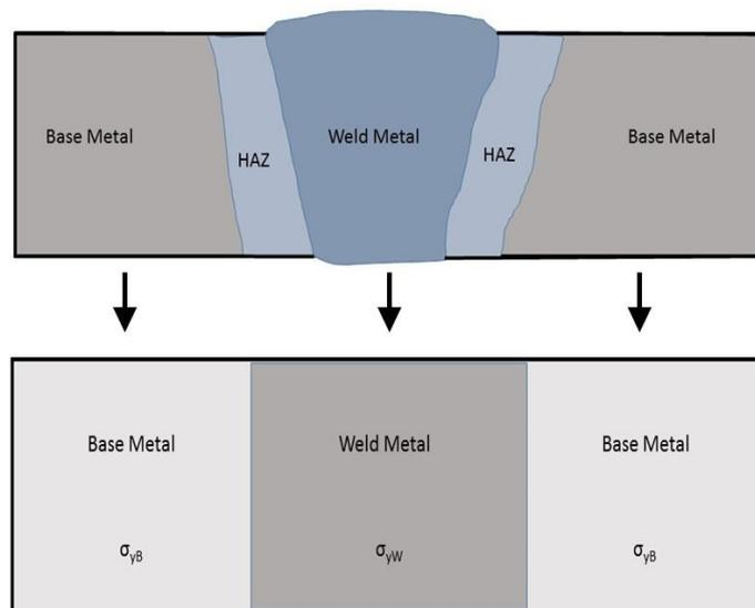
Figure 1: Weld simplification in ECA procedures: homogeneous properties and straight fusion lines
