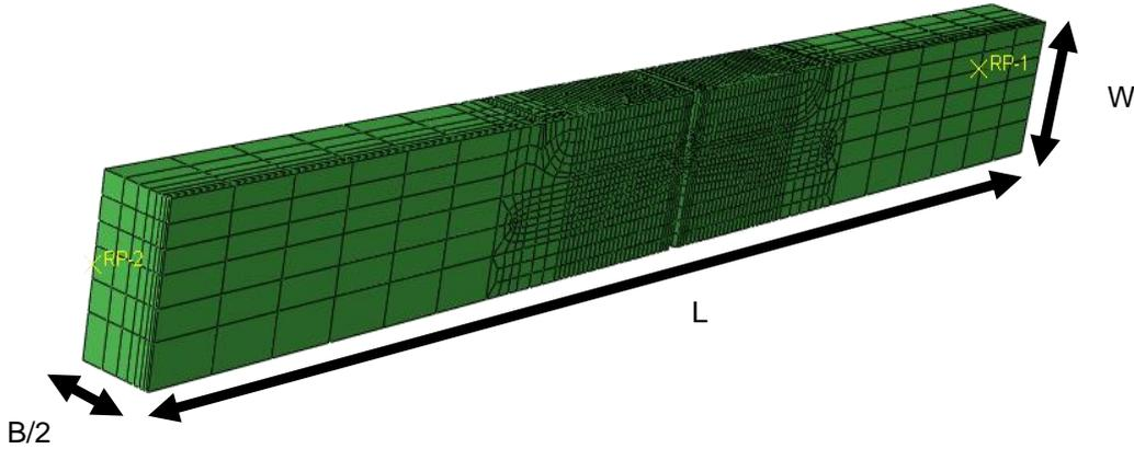
Figure 4: SENT test specimen modelled in ABAQUS with the dimensions used in the parameter description. The width is chosen only half of the real value because of symmetry as this reduces the number of calculations.
