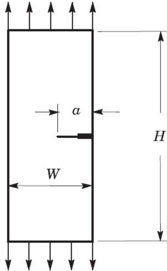
Figure 2: A SENT specimen with  $W$  the specimen width,  $H$  the specimen height and  $a$  the notch depth [5].
