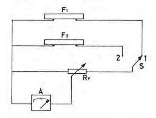
Fig. 1. The principle of the relative light intensity meter constructed by Brechtel 1962.
