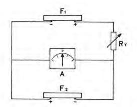
Fig. 2. The principle of a relative light intensity meter with compensating circuit.
