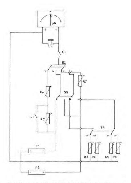
Fig. 4. The practical outline of the relative light intensity meter with compensating circuit and with possibilities for absolute measurements. S<sub>1</sub> on/out S<sub>4</sub> 20/100 f.c. S<sub>2</sub> f.c./% S<sub>5</sub> above/below S<sub>3</sub> A-/B-scale S<sub>6</sub> zero-set.
