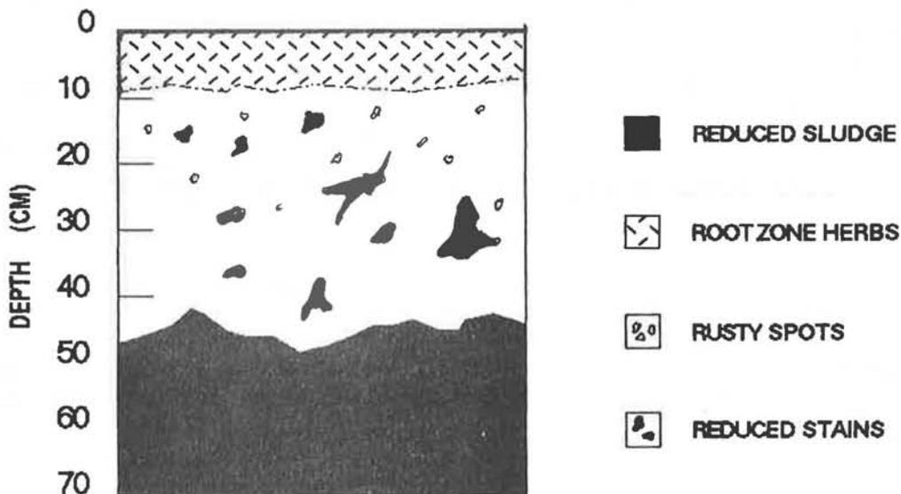
**Fig. 4** Sludge profile after 3 years of aging
