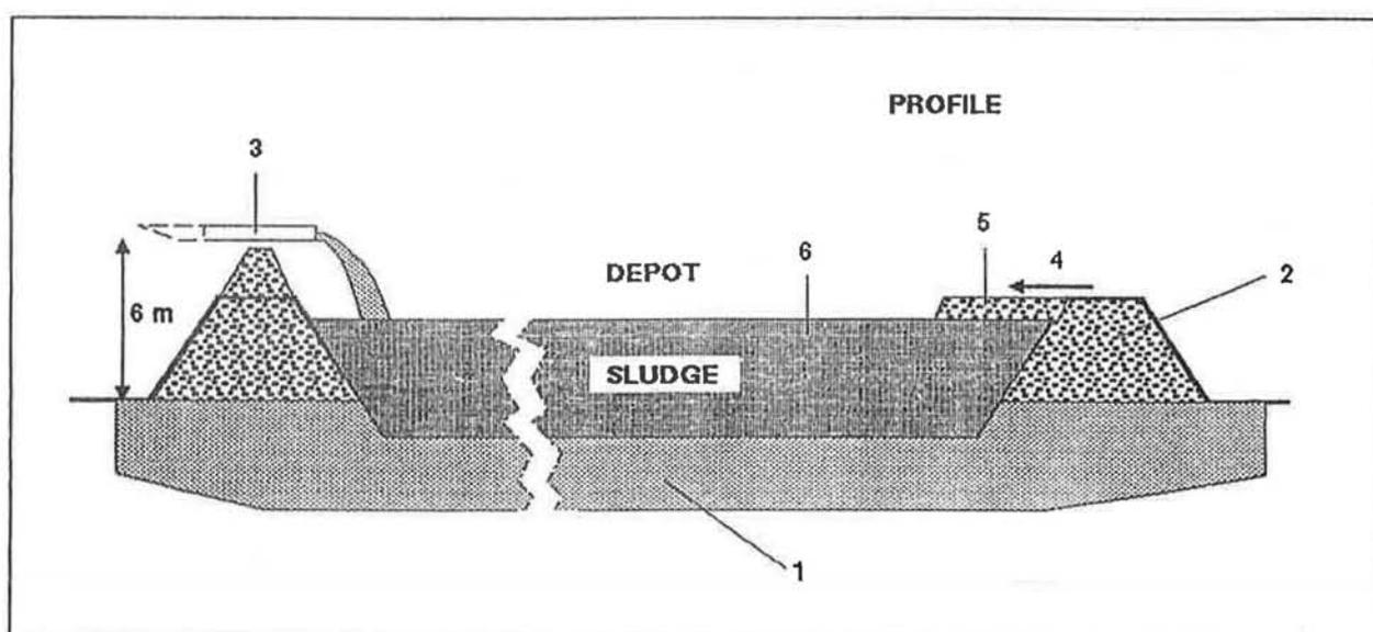
Fig. 1. Schematic vertical section of a sludge disposal basin
