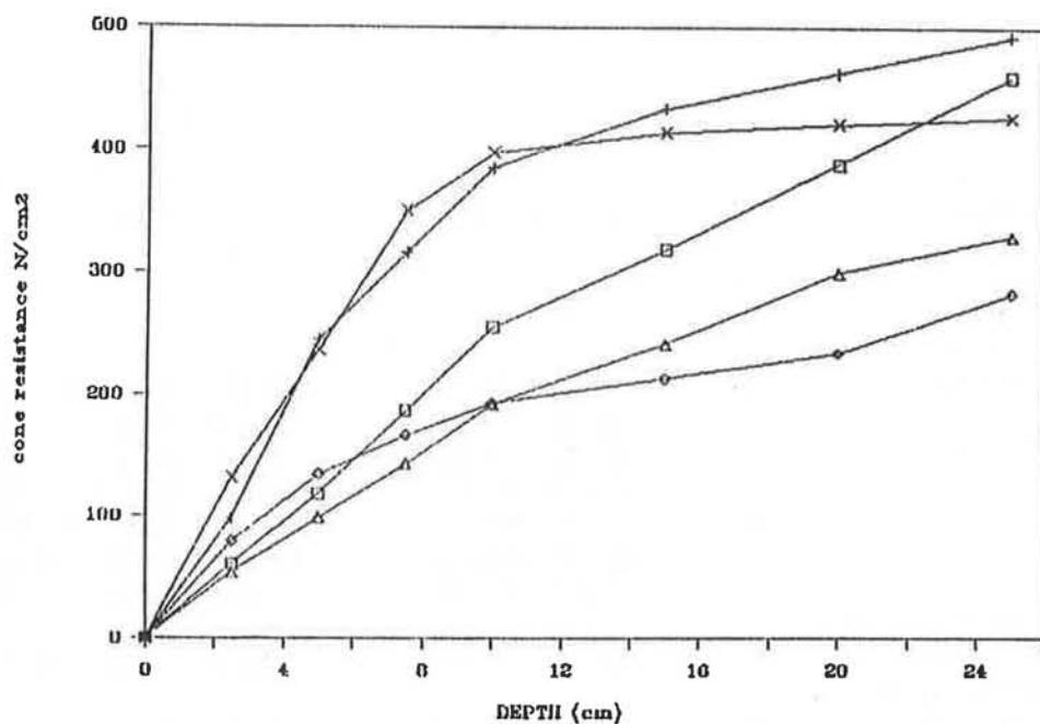
Figure 1. : Mean penetrometer cone resistance ( $N \cdot cm^{-2}$ ) as a function of depth (cm) for the investigated forest stands (Plot 1:  $\square$  limed beech,  $+$  beech; Plot 2 :  $\diamond$  maple,  $\Delta$  oak and  $\times$  beech).
