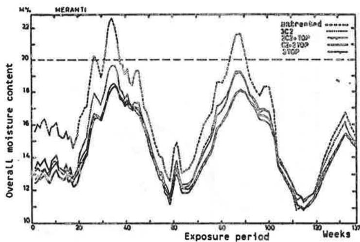
FIGURE 7: Difference in overall moisture content between treated and untreated meranti samples during 137 weeks' exposure.
