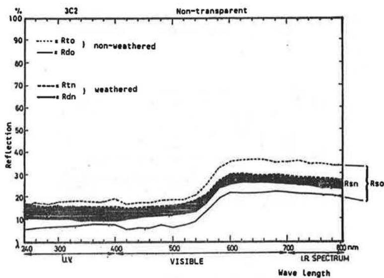
FIGURE 13: Reflectance spectra of a semi-transparent C2 + TOP-system.
