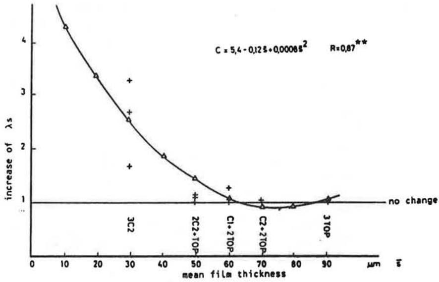
FIGURE 4: Determination of the critical film thickness  $s$ .
