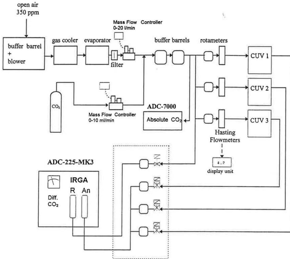
Figure 1. Schematic presentation of the phytotron of the Laboratory of Plant Ecology (Samson et al., 1997)
