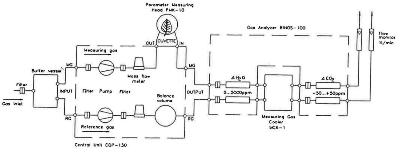
Figure 2. Schematic overview of the WALZ porometer (WALZ, 1991)
